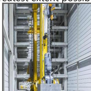
智能立体库进行硅钢存放和自动转运 Intelligent three-dimensional warehouse for silicon steel storage and automatic transportation
