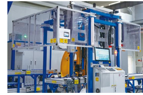
配变铁心自动试验设备 Automatic testing equipment 美变、干变铁心智能试验系统 Intelligent Test System for dry type and pad mounted cores
