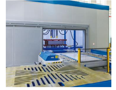
配变铁心自动试验设备 Automatic testing equipment 美变、干变铁心智能试验系统 Intelligent Test System for dry type and pad mounted cores
