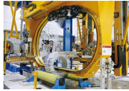
定尺条料自动绕包线 Automatic wrapping line for fixed length strip materials
