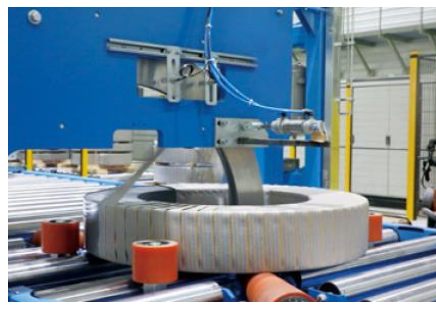
定尺条料自动绕包线 Automatic wrapping line for fixed length strip materials
